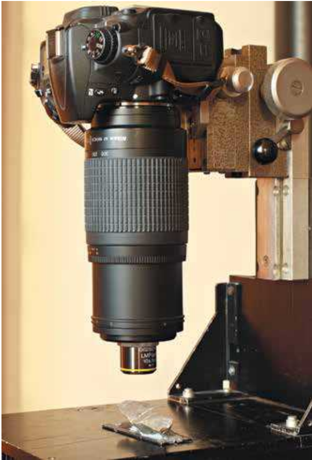
Fig. 7. Long working distance Olympus LMPlanFL 10x/0.25 microscope objective coupled to a 70–300 mm telephoto zoom lens.
