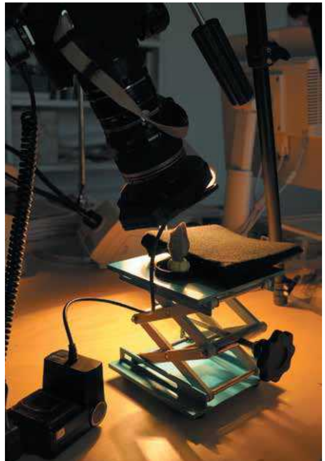
Fig. 14. Device for photogrammetric shots at macroscopic scale: Canon EOS 1000D SLR camera with a Canon EFS 60 mm f/2.8 macro objective, 7 cm macro extension tubes and a ring flash, attached to a tripod.
