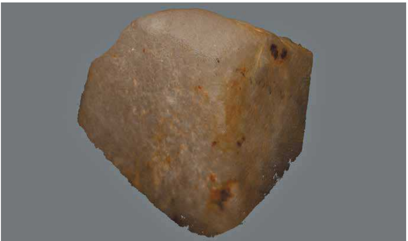
Fig. 16. Dense colored point cloud (2 830055 points) produced by Photoscan from the series of 32 views taken with the device of fig. 14 and downsampled to 3.84 MPixels before processing for compensating the low depth of field. This is a Meshlab screenshot of the point cloud, not of the meshed model, nor of the meshed and textured one.
